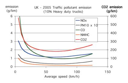
Figure 5.12. Traffic Emissions vs. Average Speed (UK DfT)
