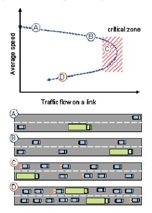
Figure 3.4. Uninterrupted Flow Speed-Flow Curve
