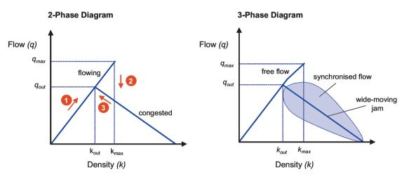
Figure 3.6. Capacity Drop Illustrated for Two-Phase and Three Phase Models
