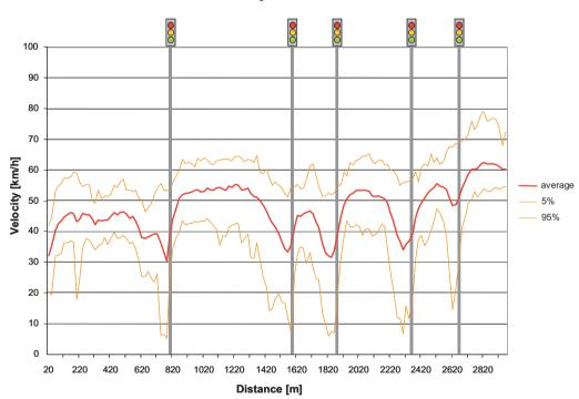
Figure 3.8. Aggregated Floating Car Data for a Section of a Signalized 2-lane Major-Road in Munich
