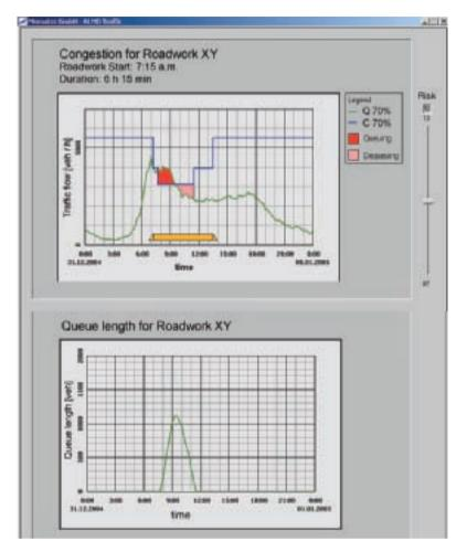
Figure 8.4. Roadwork Management System Hessen
