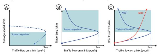
Figure 5.2. Translation of the Fundamental Speed-Flow Diagram into a Cost Function
