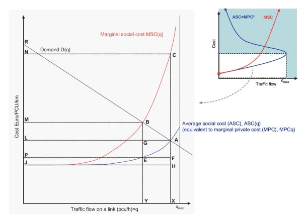
Figure 5.3. "Simplified" Diagram of Road Congestion
