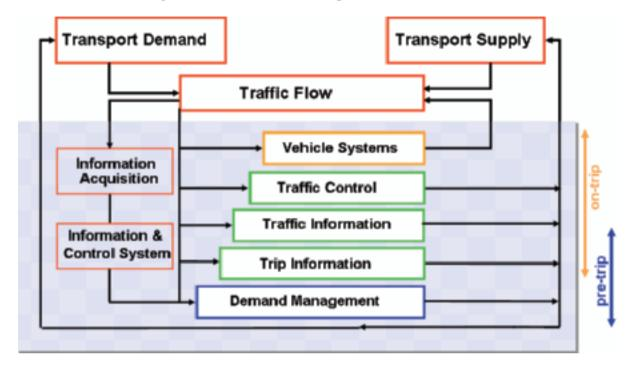
Figure 10.1. Functional Concept of ITS measures
