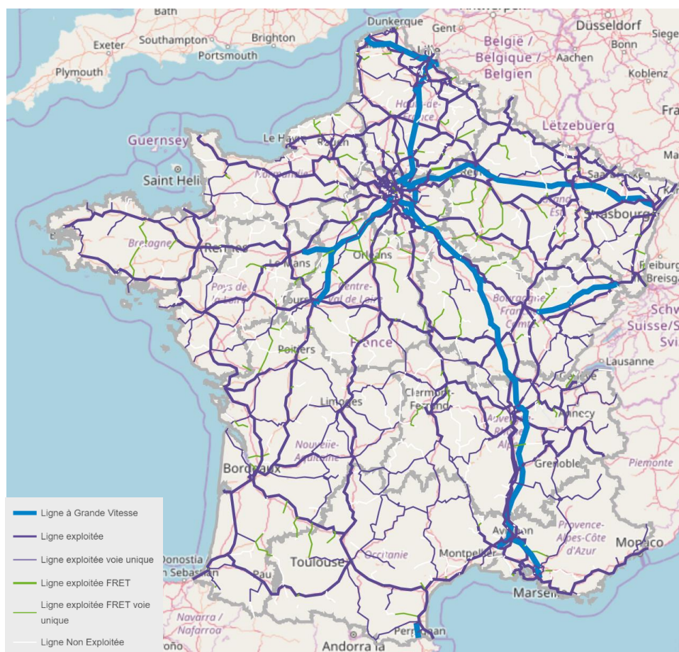
Figure 4.2. High speed rail network
