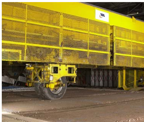
Linear fatigue machine (length 2 m)
