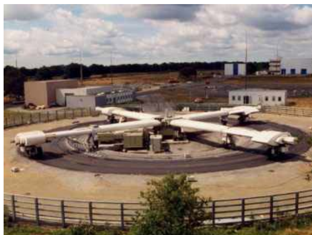
Circular fatigue carousel (diameter 20 m)
