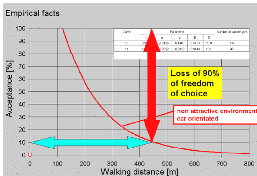
Figure 19. If the walking distance at the origin and destination of trips differs according to the various modes, as it does today, body energy consumption becomes the decisive factor for modal choice
