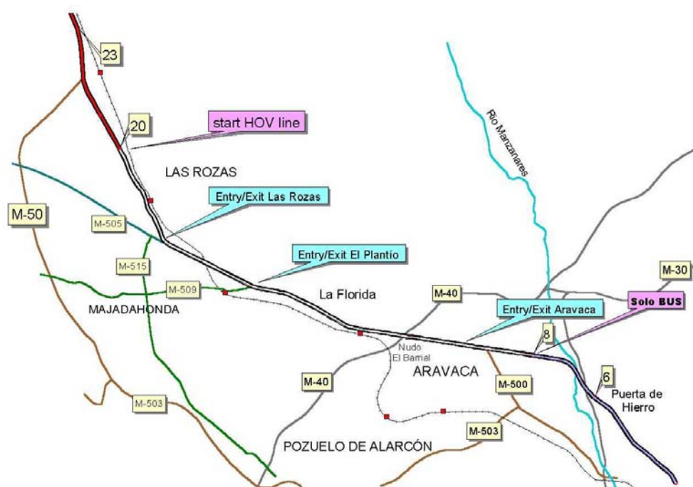
Figure 2. BUS/HOV lane: Sections and access points
