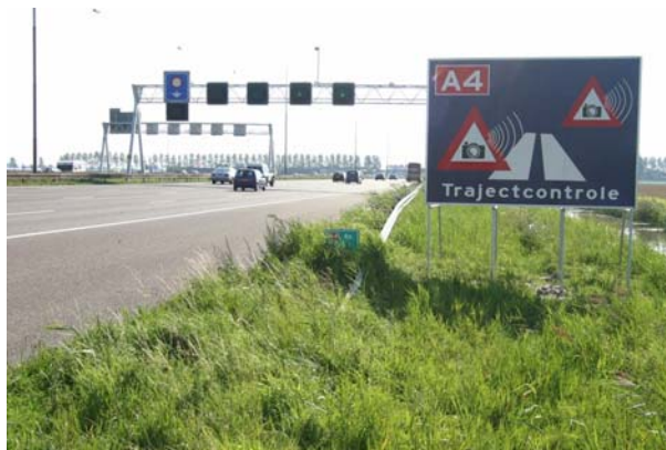
Figure 9.6. Section Control in the Netherlands
