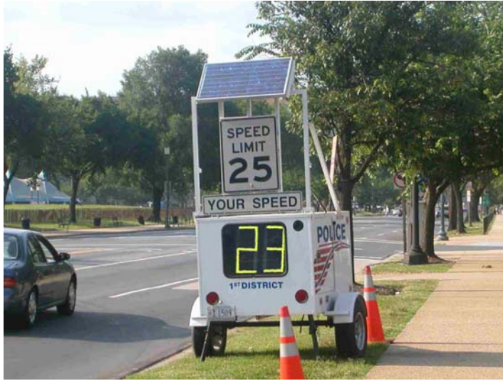
Figure 6.6. Variable message sign displaying the speed limit and the current speed of the vehicles (United States)
