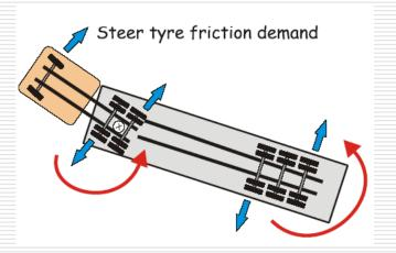
(6) **Steer Tyre Friction Demand -** The maximum friction of the steer tyres of the hauling unit in a prescribed low speed turn.
