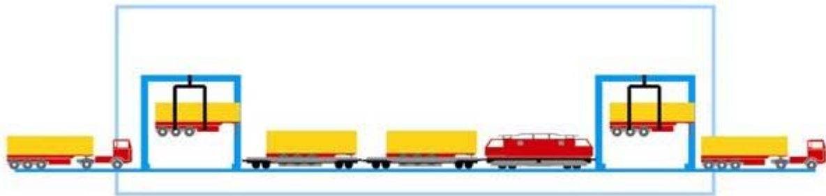
Figure 5.4. Semi-trailers are transferred between road and rail
