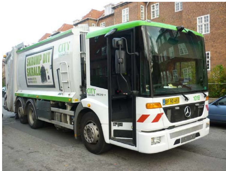
Figure 5.5 Truck with low level windscreen and side windows (Copenhagen)
