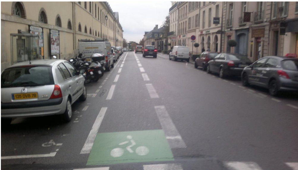
Figure 5.42 Offside cycle lane (St. Germain-en-Laye, France)
