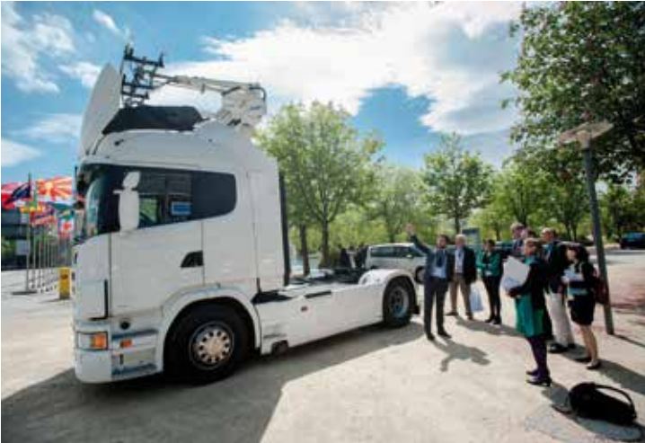
A truck with pantograph for use on Siemens' eHighways in the outdoor exhibition
