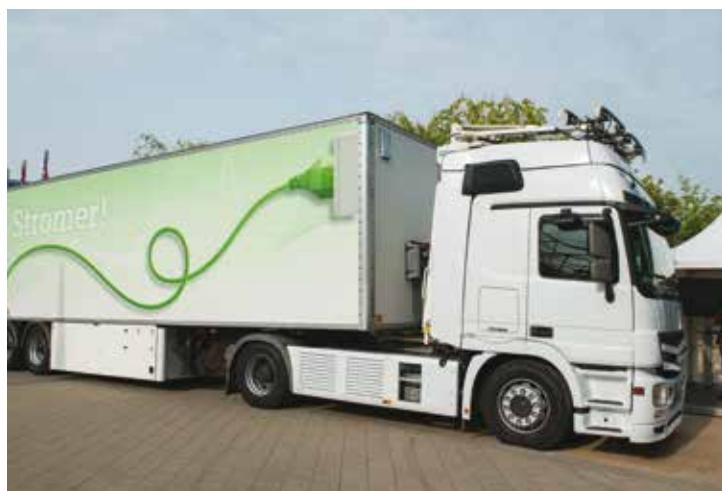
A prototype truck with pantograph for use on the Siemens eHighway outside the Leipzig conference centre
