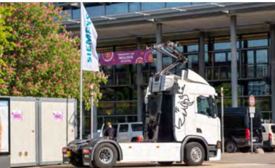
A pantograph-equipped electric truck for use on "eHighways" developed by Siemens stands outside the venue
