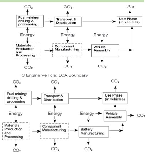
PHEV Vehicle: LCA Boundary
