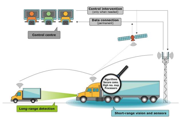
The three main components of a fully automated truck's potential operating environment are its on-board systems, supporting infrastructure and the (remote) control centre. As noted above, fully autonomous vehicles would require less supporting ICT infrastructure, but that puts much stronger emphasis on the on-board systems.
