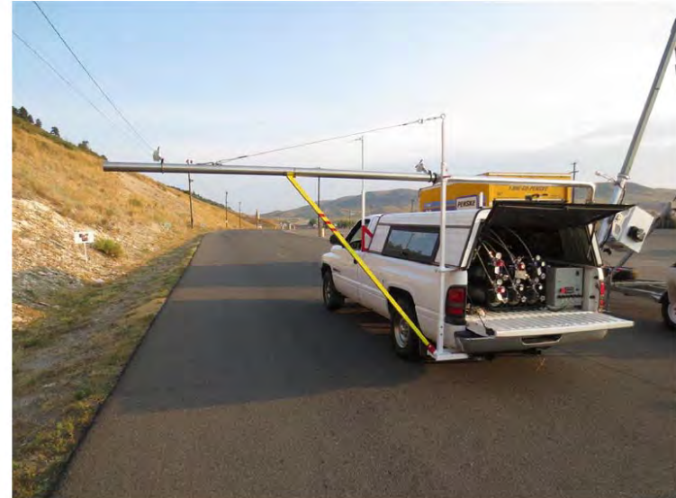
Figure 2. RSD Audit Truck with Engine Exhaust 10-foot Side Extension
