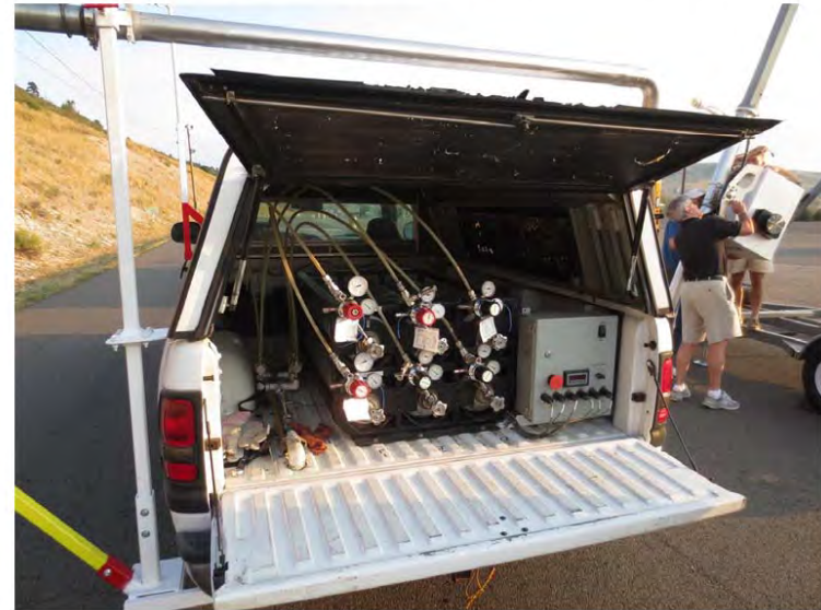
Figure 2. RSD Audit Truck with Engine Exhaust 10-foot Side Extension
