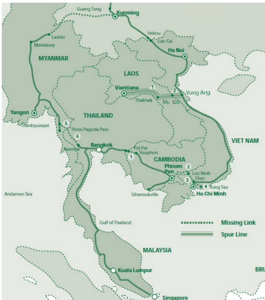
Figure 6. The 2010 Singapore Kunming Rail Link (SKRL) network and missing links
